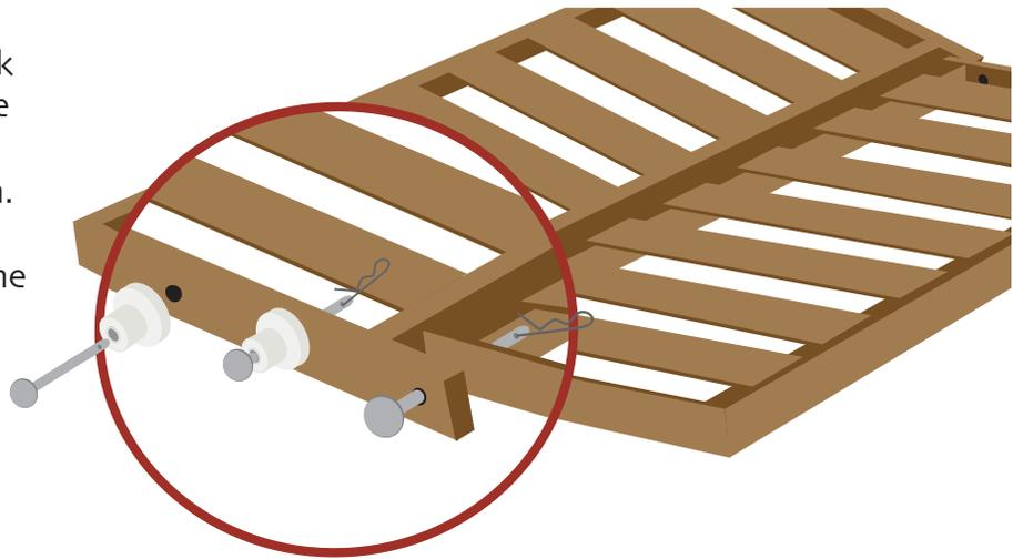
**3** Lower the assembled deck into the frame as shown. Line up the slide rollers to the grooves in the arms. The top rollers fits into the vertical grooves and the lower rollers fits into the horizontal grooves.
