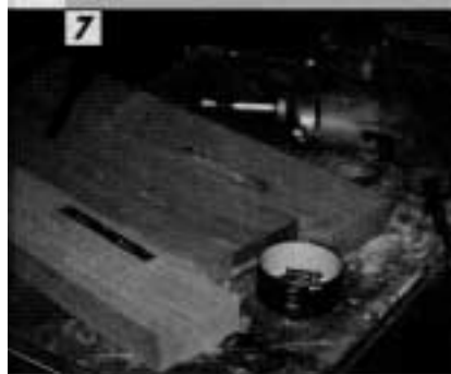
7 The female part of the bed-rail connector is mortised into the sofa leg. Each bed-rail part must be fitted and labeled for its position (see text). 8 Lay out the track routing template carefully. Bore the 1-1/2-in.-dia. holes first. Then cut away most of the waste with a sabre saw. Be careful to stay
