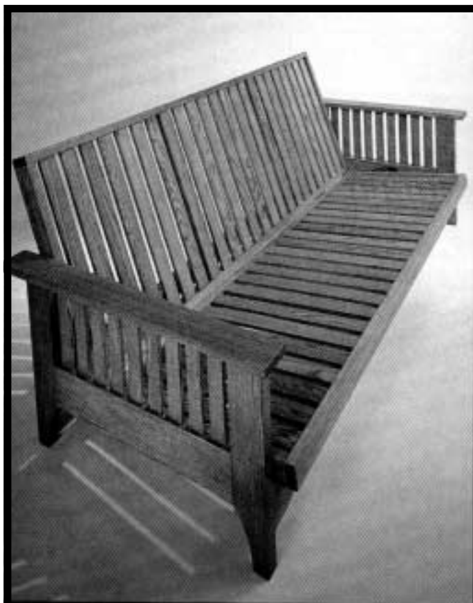
With the cushion removed, the ribs are revealed. They provide plenty of strength for a heavy load, but because they're not too thick (1/2 in.), they're also flexible. Note that the hinges barely protrude above the surface.
