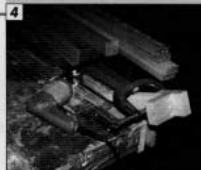
4 Make a drill bushing on the drill press to accurately locate the three dowel holes at each corner of the seat frame and back frame. Use stock of the same width as the parts to ensure alignment. 5 The maple tracking pins are wedged and glued into their holes. Be sure the wedge kerf in the pin
